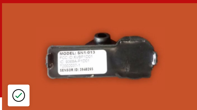
TPMS sensor in an acceptable condition
