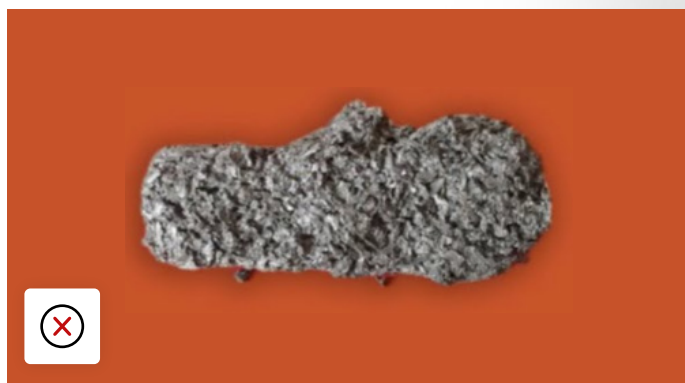
TPMS sensor contaminated by sealant
